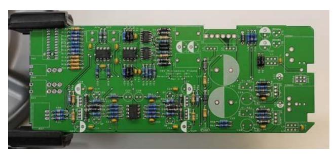
**11.** Install the ferrite filters now. These parts are not polarized and can be installed in either direction.
