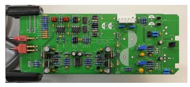
22. Add electrolytic capacitors C4, C7, C39 and C40. Again, electrolytic capacitors are polarized and must be installed the right way around! Be absolutely sure to observe the correct polarity when installing these parts. Add polypropylene capacitors C5 and C6 as well.
