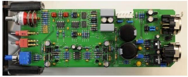
**29.** Before going on to initial power-up, carefully check your work. Make sure you haven't created any solder bridges between pads, or between a pad and the ground plane.
