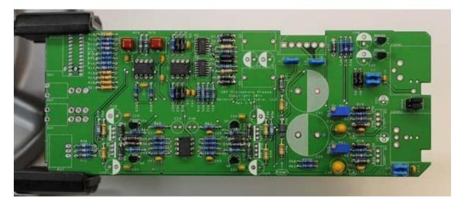
18. Add the short electrolytic capacitors now. C23 and C30 are not polarized, but the rest are and must be installed the right way around! Be absolutely sure to observe the correct polarity when installing these parts. The negative leads of the electrolytic caps are marked with a colored stripe. The positive pads on the circuit board are marked with a small "+" sign.
