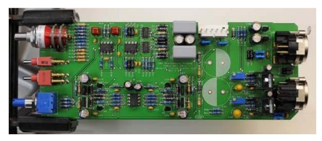
28. Install the bulk filter capacitors C31 and C35. Push them in firmly until they are fully seated against the board. Again, electrolytic capacitors are polarized and must be installed the right way around! Be absolutely sure to observe the correct polarity when installing these parts.
