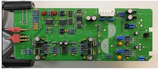
**23.** Add large capacitors C5 and C6. Be sure to not overheat the leads, as these parts are susceptible to damage from excess soldering heat.
