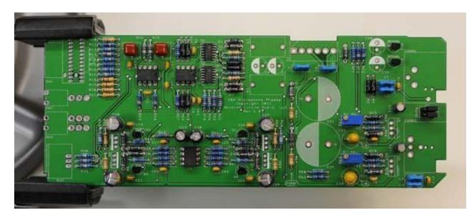
19. Add transistors Q5, Q6, Q9, and Q10. Make sure to install the transistors correctly! These parts are not the same and are not interchangeable. The heavy line on the silkscreen outline indicates the back of the transistor, the side without markings. Make absolutely sure you don't insert them backwards.
