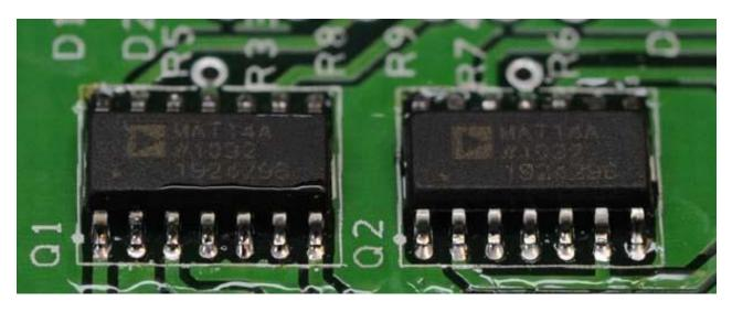
10. Install U1, U2, and U3 now. Pay close attention to the IC markings. Align the notch on the IC with the notch on the silkscreen outline! IC sockets are not included in the kit and are not recommended. Socketing the ICs will interfere with the ability of the PC board to conduct heat away from the parts.
