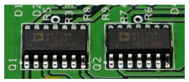
9. Flow solder onto the rest of the pads. Use a flux pen or liquid flux for best results.
