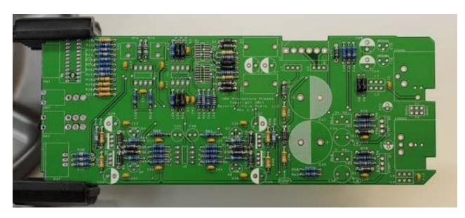
**7.** Install Q1 and Q2 now. Start by flowing a small amount of solder on two pads only as shown.
