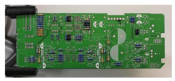
5. Next, add the protection diodes D1 through D19. Diodes are polarized and must be installed the right way around! The colored band on the diode matches the white band on the silkscreen.
