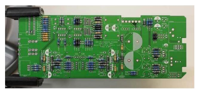
6. Add the small ceramic capacitors. These capacitors are not polarized and can be installed in either direction, but pay close attention to the capacitor markings! These parts all look alike, but they are not interchangeable. Putting one in the wrong spot will not prevent the preamp from passing signal, but it can seriously impair its performance.
