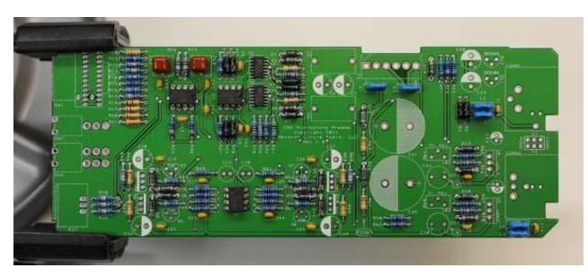
14. Add small transistors Q3, Q4, Q7, and Q8. These parts are not the same and are not interchangeable. Align the flat side of the transistors with the flat side of the silkscreen outline.
