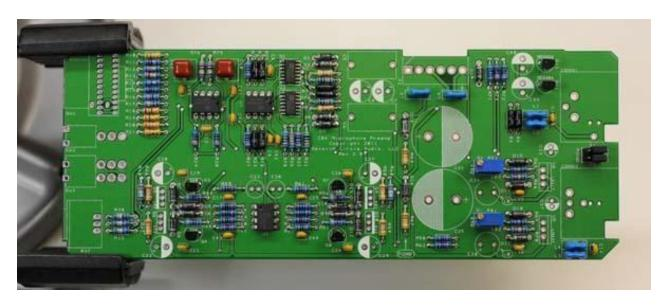
17. Add tantalum capacitors C34 and C38. Tantalum electrolytic capacitors are polarized and must be installed the right way around! Be absolutely sure to observe the correct polarity when installing these parts. The positive leads of the tantalum caps are marked with a small "+" sign. The positive pads on the circuit board are marked with a small "+" sign.
