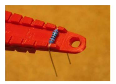
4. Insert the 1/4-watt resistors. Check the Bill of Materials (BOM) for help in reading the resistor color bands. It's also a good idea to actually measure each resistor with your DMM as you place it on the board, just in case you've decoded it incorrectly. Don't rely on the photos for component placement. THE PCB PICTURES ARE NOT NECCESARILY THE CURRENT REVISION! If the resistor value silk-screened on the board doesn't agree with the value on the schematic or parts list, follow the schematic.
