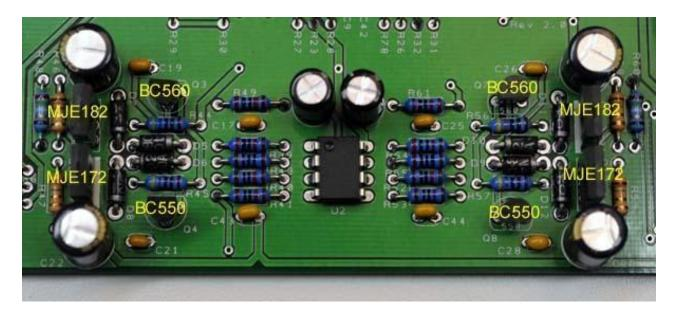
**15.** Add Q11 and Q12. Again, these parts are not the same, and are not interchangeable. **Align the flat side of the transistors with the flat side of the silkscreen outline.**
