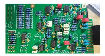
**9.** Install the blue EMI filters now. These parts are not polarized and can be installed in either direction.
