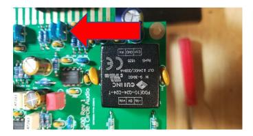
10. Install the film caps. These parts are not polarized and can be installed in either direction.
