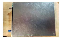
5. Attach faceplate using the nuts, but NOT the washers! Add knobs to the front
