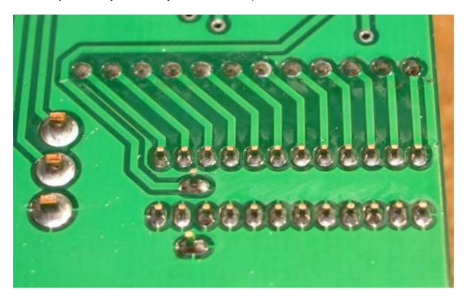
**15.** Add all of the DC-DC power converter parts to the board. Make sure they're fully seated before soldering.
