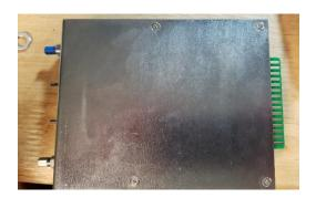
4. Install cover using 4 small flathead screws.
