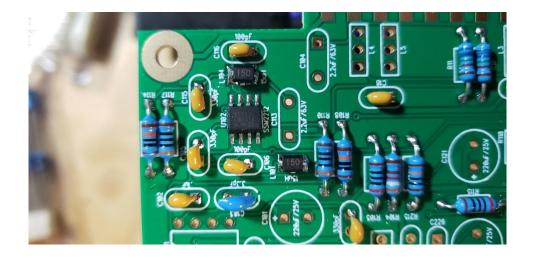
8. Install all other 8-pin IC's now. Pay close attention to the IC markings. Align the notch on the IC with the notch on the silkscreen outline! IC sockets are not included in the kit and are not recommended. Socketing the ICs will interfere with the ability of the PC board to conduct heat away from the parts.
