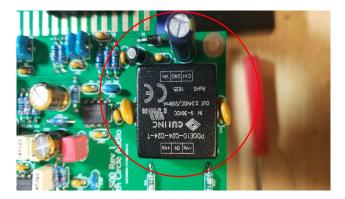
**16.** Before going on to initial power-up, carefully check your work. Make sure you haven't created any solder bridges between pads, or between a pad and the ground plane.
