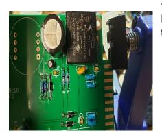
**17.** Install the parts for the power supply. The DC/DC converter, caps, and Inductor. Be extra careful to not leave solder shorts on these parts!
