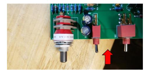
11. Install C18 and C19, the phantom power filter caps. Aluminum electrolytic capacitors are polarized and must be installed the right way around! Again, be absolutely sure to observe the correct polarity when installing these parts. The negative leads of the electrolytic caps are marked with a colored stripe. The positive pads on the circuit board are marked with a small "+" sign.
