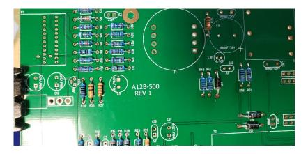
5. Next, add the protection diodes D11, D13, and D14. Diodes are polarized and must be installed the right way around!
