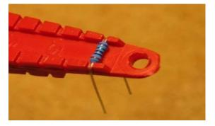
4. Install the 1/4-watt resistors. Check the Bill of Materials (BOM) for help in reading the resistor color bands. It's also a good idea to actually measure each resistor with your DMM as you place it on the board, just in case you've read it wrong. Don't rely on the photos for component placement. If the resistor value silk-screened on the board doesn't agree with the value on the schematic or parts list, follow the schematic
