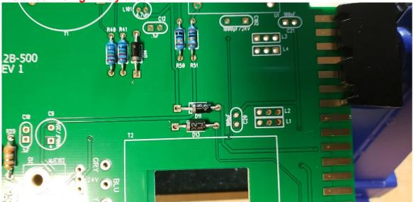
6. Add the glass diodes D1-D6. The colored band on the diode matches the white band on the silkscreen. Diodes are polarized and must be installed the right way around!
