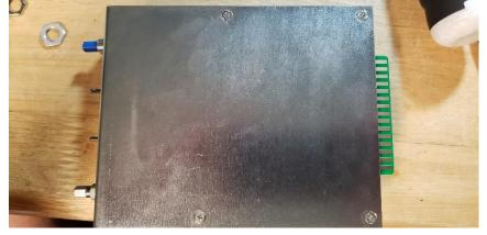
4. Install cover using 4 small flathead screws.
