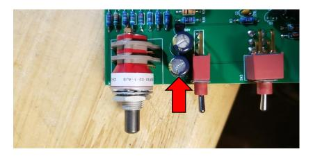
**12.** Attach gain trim control R1. Make sure the control is seated flat to the board before soldering the leads. You may want to add a small dab of silicone adhesive to the bottom of the control to hold it more securely.
