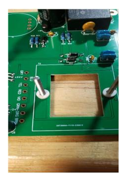
**16.** Solder the transformer leads to the circuit board as shown. The wire color is silk-screened next to each pad. The leads should not cross over and should be trimmed to the length shown. Do not leave the leads un-trimmed. **GRAY**,
