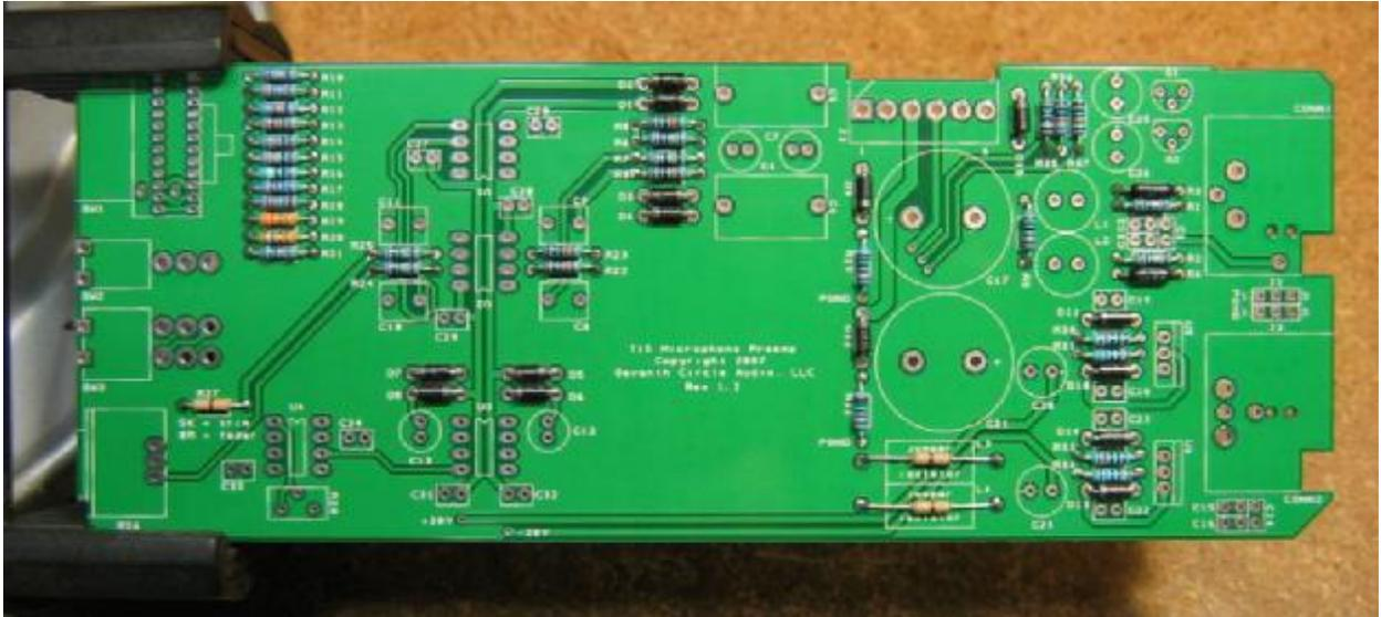
5. Next, add the protection diodes D1 through D15. **Diodes are polarized and must be installed the right way round!** The colored band on the diode matches the white band on the silkscreen.
