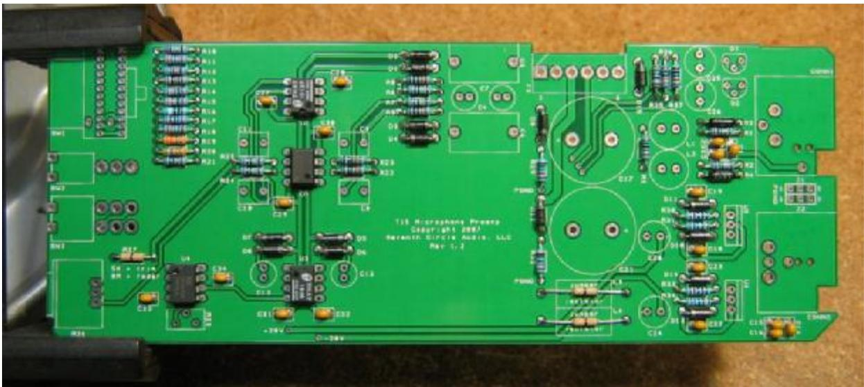
8. If you need to drive extremely long cables (greater than 50m) or know that you'll be connecting the preamp to capacitive loads (you probably won't), add the "load isolator" inductors at L3 and L4. Otherwise, solder jumpers in their place as shown. **You must install either the JT-OLI-3 inductors or jumpers at L3 and L4. Otherwise, the preamp will not pass a signal!**
