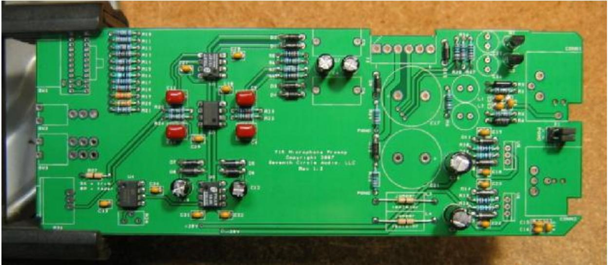
14. Install L1 and L2. These parts may have markings that are hard to read or be completely unmarked. You can verify that they're inductors by measuring their resistance, which should be very low. These parts are not polarized and may be installed in either direction.
