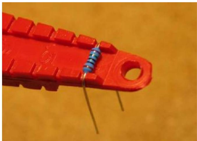
4. Insert the 1/4-watt resistors. Check the Bill of Materials (BOM) for help in reading the resistor color bands. It's also a good idea to actually measure each resistor with your DMM as you place it on the board, just in case you've read it incorrectly. Don't rely on the photos for component placement. If the resistor value silk-screened on the board doesn't agree with the value on the schematic or parts list, follow the schematic.
