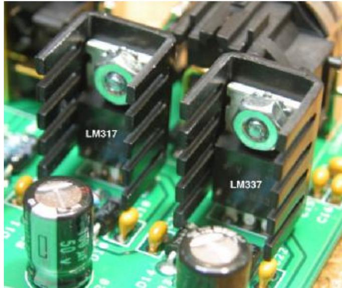
25. Install the bulk filter capacitors C17 and C21. Push them in firmly until they are fully seated against the board. Again, **electrolytic capacitors are polarized and must be installed the right way round!** Be absolutely sure to observe the correct polarity when installing these parts.
