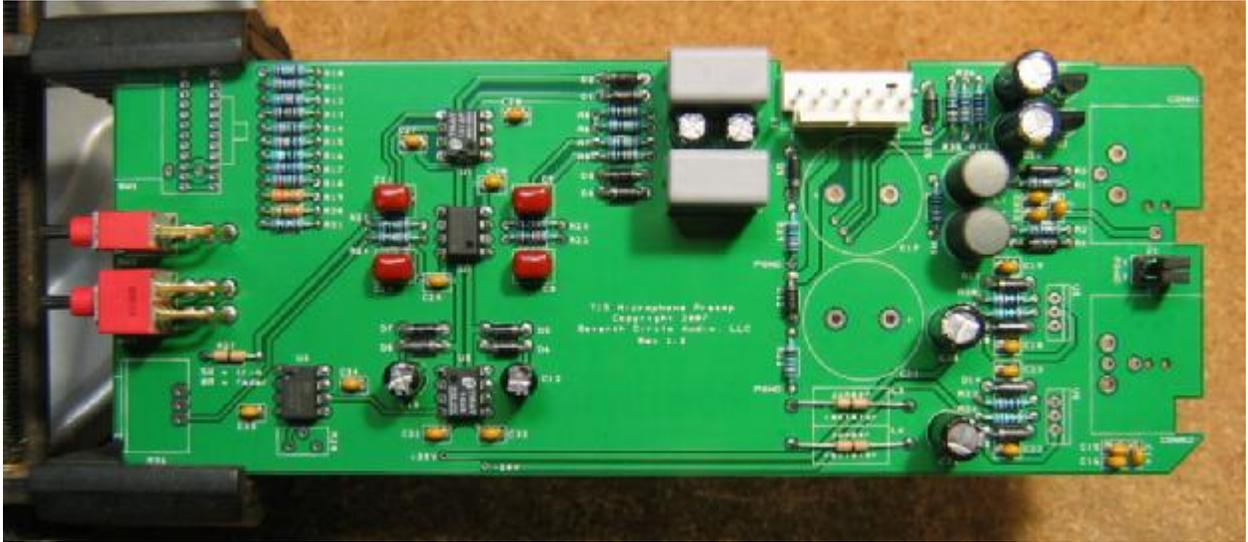
18. Attach gain trim control R26. Make sure the control is seated flat to the board before soldering the leads. You may want to add a small dab of silicone adhesive to the bottom of the control to hold it more securely.
