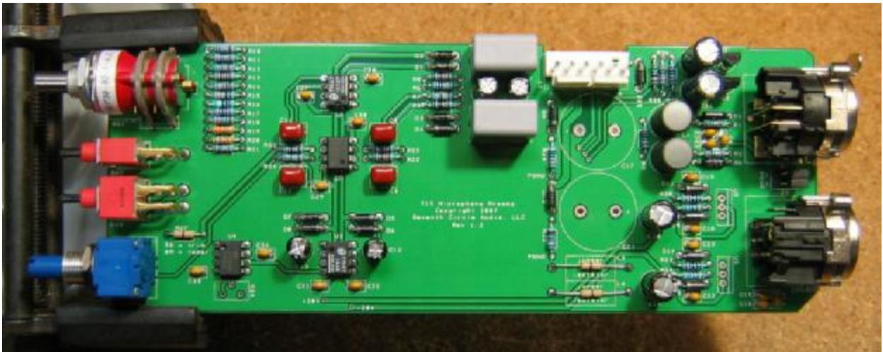
24. Using the hardware supplied, attach heat sinks to U5 and U6 and solder them in place. **Make sure to install the regulators correctly!** These parts are not the same, and are not interchangeable.
