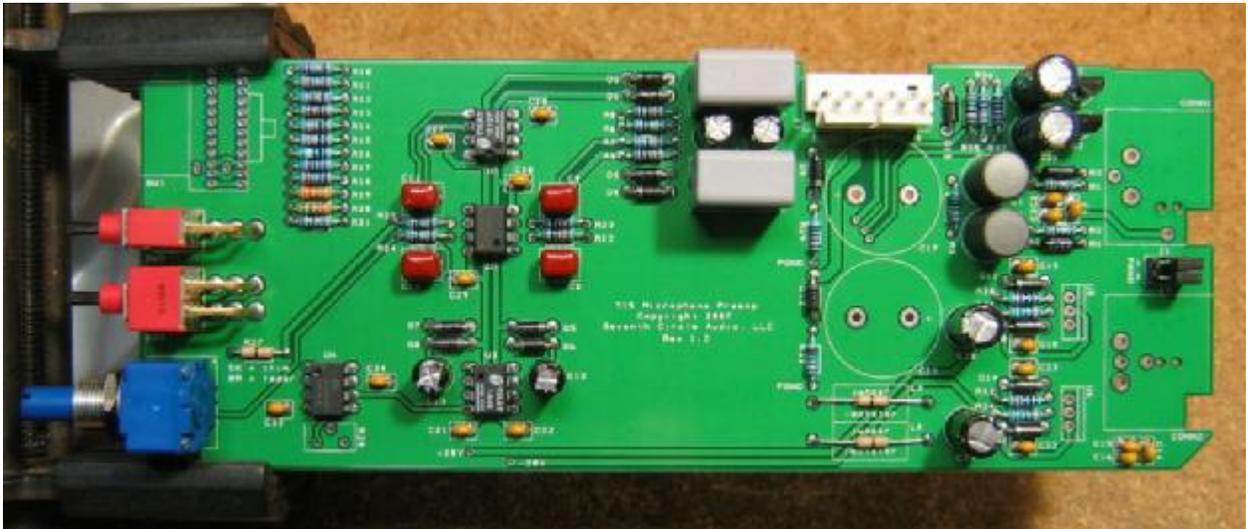
19. Insert the stop pin in rotary switch SW1 at the position shown. Push the pin in completely.
