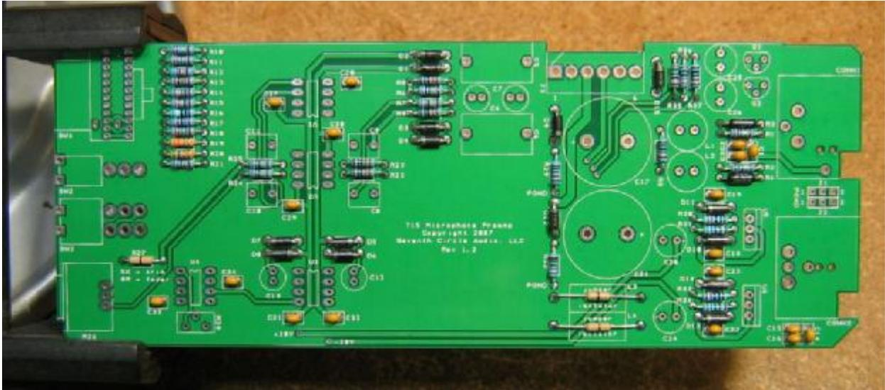
7. Install U1 through U4 now. **Pay close attention to the IC markings. Align the notch on the IC with the notch on the silkscreen outline!** If you'd like the option of easily swapping or replacing the ICs, now is the time to add the sockets. **Sockets are optional and are not included in the kit.**
