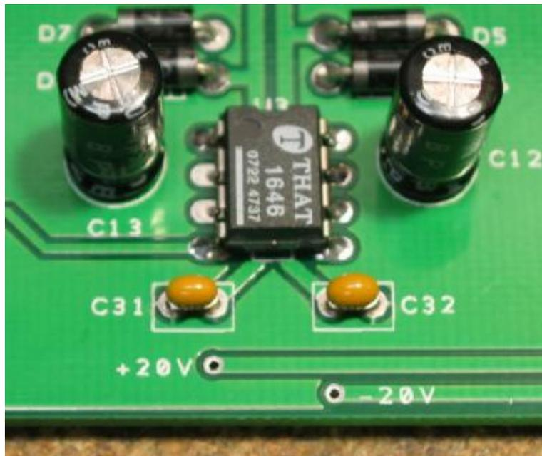
30. With the negative probe still at **PGND**, measure the voltage at U1, pin 4 or the **-20V** pad shown above. You should measure very close to -18V.
