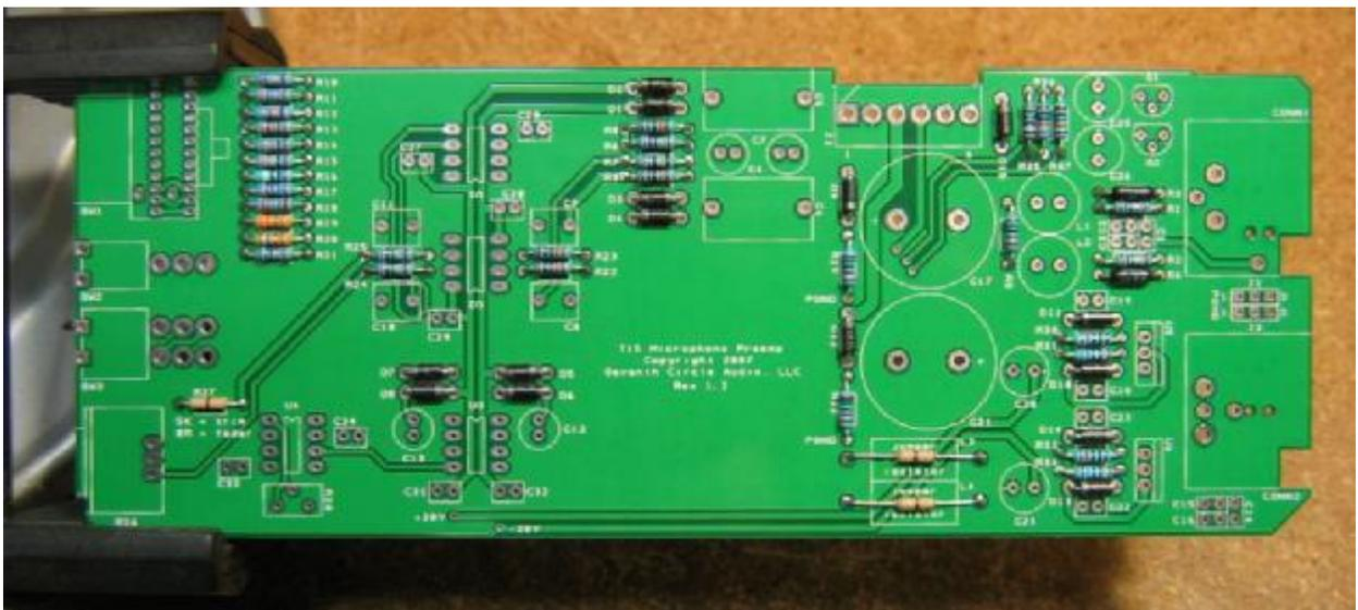
6. Add the 470pF and 0.1uF ceramic capacitors. These capacitors are not polarized and can be installed in either direction, **but pay close attention to the capacitor markings!** These parts look alike, but they are not interchangeable. Putting one in the wrong spot will not prevent the preamp from passing signal, but it can seriously impair its performance.
