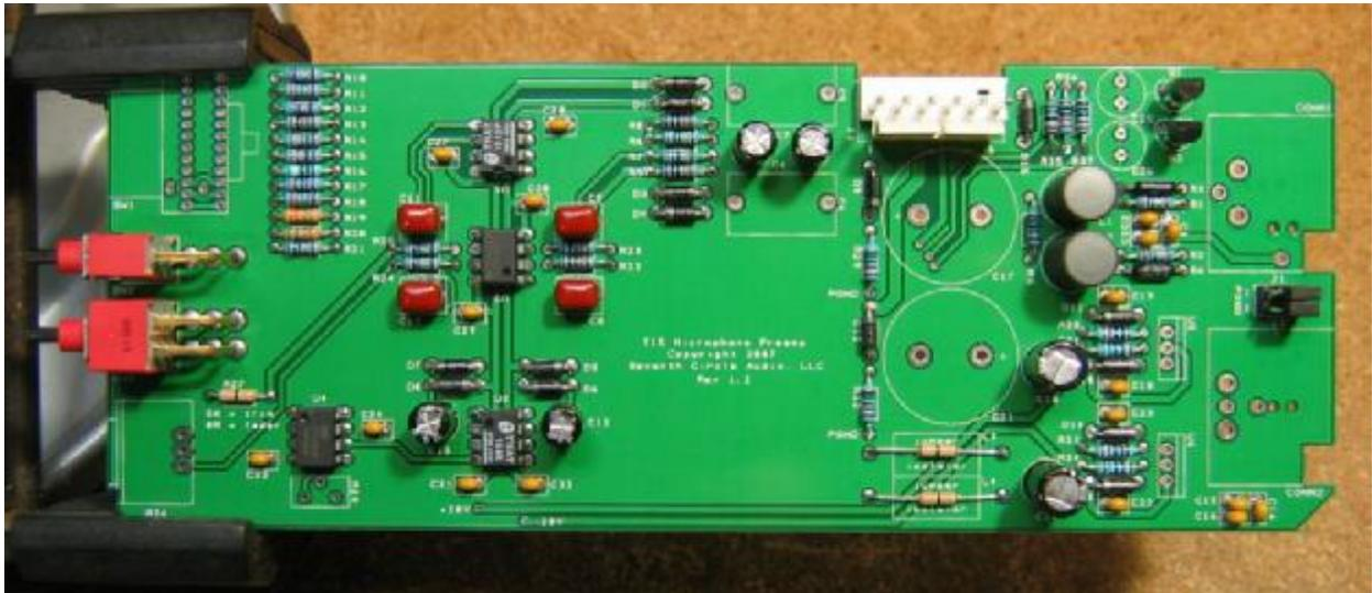
17. Add electrolytic capacitors C25 and C26. Again, **electrolytic capacitors are polarized and must be installed the right way round!** Be absolutely sure to observe the correct polarity when installing these parts. Add polypropylene capacitors C5 and C6 as well.
