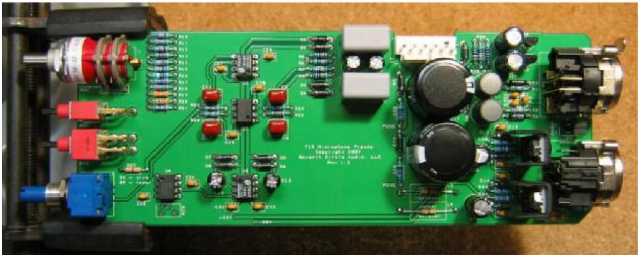
26. Before going on to initial power-up, carefully check your work. Make sure you haven't created any solder bridges between pads, or between a pad and the ground plane.
