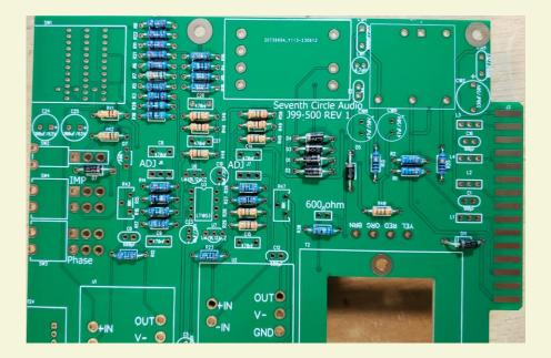
6. Add small, yellow ceramic capacitors These capacitors are not polarized and can be installed in either direction, but pay close attention to the capacitor markings! Add blue EMI filters L1 through L6. These parts are not polarized and can be installed in either direction.
