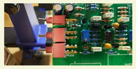
**16.** Attach gain trim control R24. Make sure the control is seated flat to the board before soldering the leads. You may want to add a small dab of silicone adhesive to the bottom of the control to hold it more securely, but it isn't necessary.
