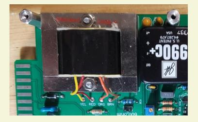
24. That's it for PCB assembly! Before going on to initial power-up, carefully check your work. Make sure you haven't created any solder bridges between pads, or between a pad and the ground plane.
