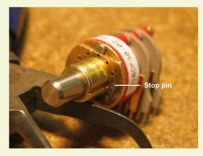
**18.** Secure the pin with the adhesive foil supplied.
