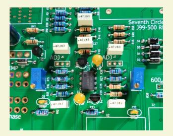
12. Add Q7, U6 and U7. Be sure to install semiconductors correctly! These parts are not the same and they are not interchangeable. Read the markings carefully and orient the packages according to the silkscreen outlines. Don't mix up the positive and negative regulators and the transistor!
