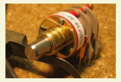
**19.** Make sure the switch is fully seated and solder it to the board. Try to make your solder joints as neat as possible, and don't use too much solder.
