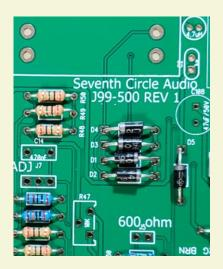
5. Insert the 1/4-watt resistors. Check the Bill of Materials (BOM) for help in reading the resistor color bands. It's a good idea to actually measure each resistor with your DMM as you place it on the board, just in case you've read it incorrectly. Don't rely on the photos for component placement. If the resistor value silk-screened on the board doesn't agree with the value on the schematic or parts list, follow the schematic.
