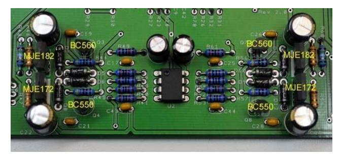
14. Add Q11. (Q12 IS NO LONGER NEEDED!) Again, these parts are not the same, and are not interchangeable. Align the flat side of the transistors with the flat side of the silkscreen outline.
