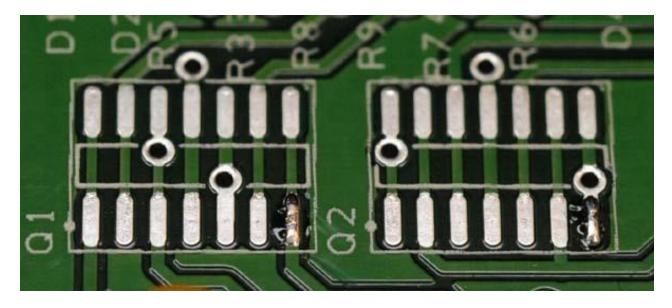
8. Carefully position the part over the pads and re-flow the solder to tack it in place. Pay close attention to the IC markings. Align the dot on the IC with the dot on the silkscreen outline!
