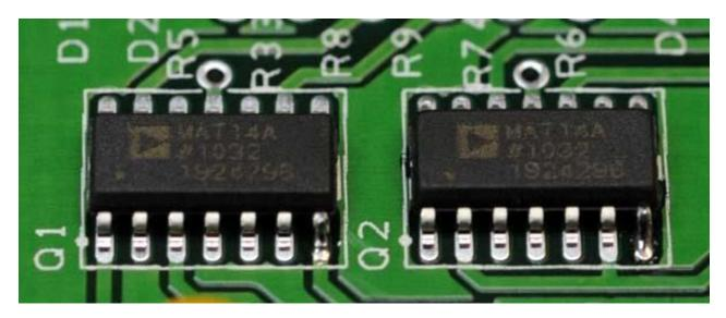
9. Flow solder onto the rest of the pads. Use a flux pen or liquid flux for best results.
