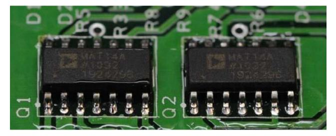
10. Install U1, U2, and U3 now. Pay close attention to the IC markings. Align the notch on the IC with the notch on the silkscreen outline! IC sockets are not included in the kit and are not recommended. Socketing the ICs will interfere with the ability of the PC board to conduct heat away from the parts.
