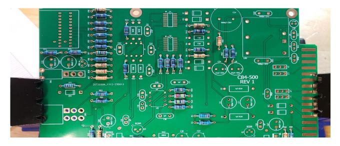
5. Next, add the protection diodes D1 through D19. Diodes are polarized and must be installed the right way around! The colored band on the diode matches the white band on the silkscreen.
