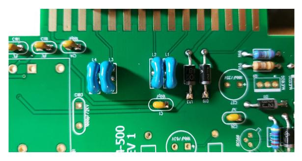
**12.** Install the 1uF film caps at C10 and C11. These parts are not polarized and can be installed in either direction.
