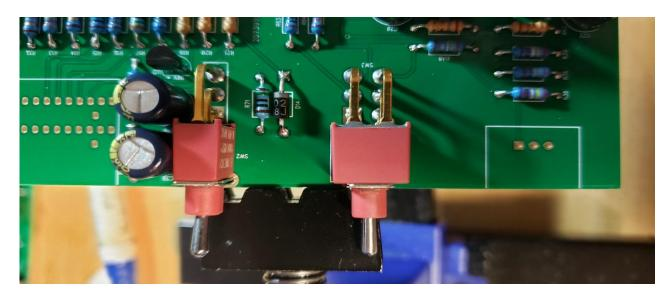
**19.** Add large capacitors C5 and C6. Be sure to not overheat the leads, as these parts are susceptible to damage from excess soldering heat.
