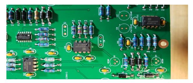
**11.** Install the blue filters, L1-L4, now. These parts are not polarized and can be installed in either direction.
