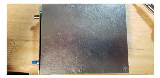
5. Attach faceplate using the nuts, but NOT the washers! Add knobs to the front
