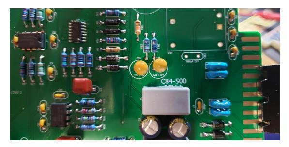
16. Add electrolytic capacitors now. C23 and C30 are not polarized, but the rest are and must be installed the right way around! Be absolutely sure to observe the correct polarity when installing these parts. The negative leads of the electrolytic caps are marked with a colored stripe. The positive pads on the circuit board are marked with a small "+" sign.
