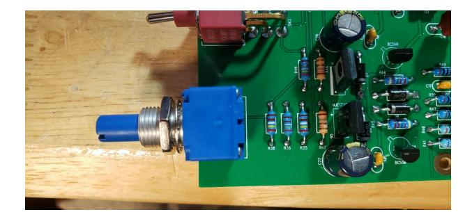
**22.** Install the bulk filter capacitor C24 as well as other power supply parts. Be EXTRA CAREFUL not to leave solder shorts on these components!
