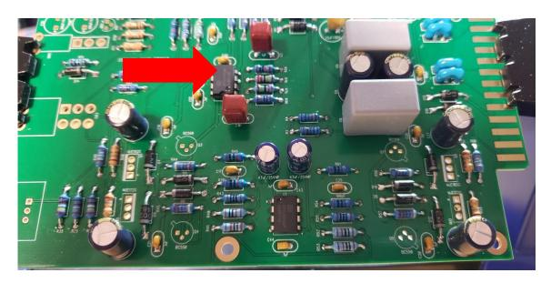
**13.** Add small transistors Q3, Q4, Q7, and Q8. These parts are not the same and are not interchangeable. Align the flat side of the transistors with the flat side of the silkscreen outline.
