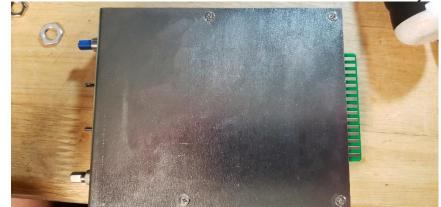
3. Use 4 small flat head screws to secure PCB to bottom tray.
