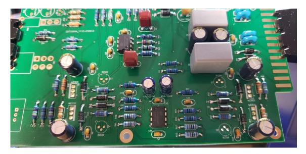
17. Add transistors Q5, Q6, Q9, and Q10. Make sure to install the transistors correctly! These parts are not the same and are not interchangeable. The heavy line on the silkscreen outline indicates the back of the transistor, the side without markings. Make absolutely sure you don't insert them backwards.
